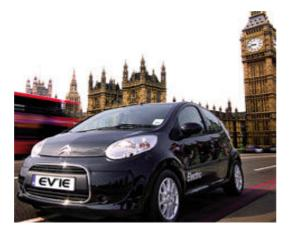
The C1 ev'ie can be fully charged in 6-7 hours from a domestic 13 amp socket at a cost of around 90p and it has a range of 60-70 miles.
